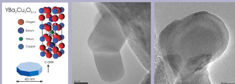
**Fig. 1:** Left: A schematic of the YBCO unit cell, and a schematic of an YBCO nanoparticle. Center: TEM image of an YBCO nanoparticle. The bar is 10 nm. Right: TEM image of an YBCO nanoparticle. The bar is 50 nm.
