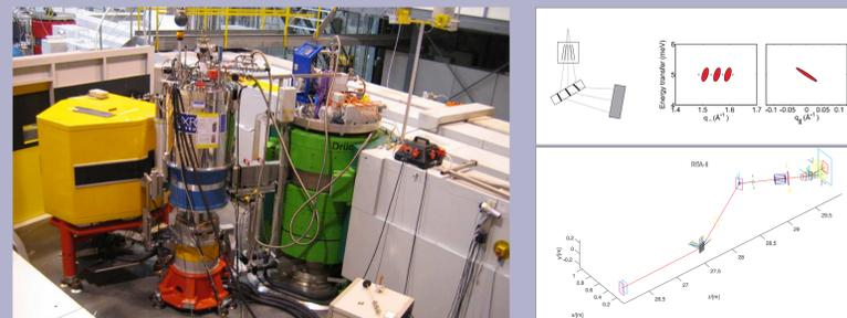
**Fig. 2:** Left: Image of the RITA-II spectrometer. From the left, the yellow detector tank containing the analyzer assembly and the PSD. The sample is located further right, inside the blue cryo magnet. The monochromator is located inside the green tank. The grey box to the right of the monochromator tank contains the neutron guide. Top-right: A schematic of the RITA-II analyzer setup. Also shown is a resolution function for a multi blade mode (3 blades). Bottom-right: A schematic of RITA-II.
